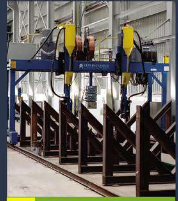
3. WELDING GANTRY + SAW MACHINE
